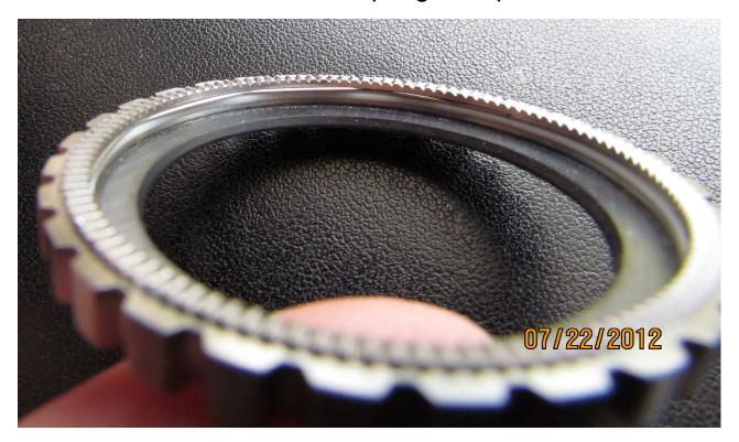
Make sure the bezel click spring is properly installed on the case. There is a "foot" on the spring that will fit into a hole in the case.
