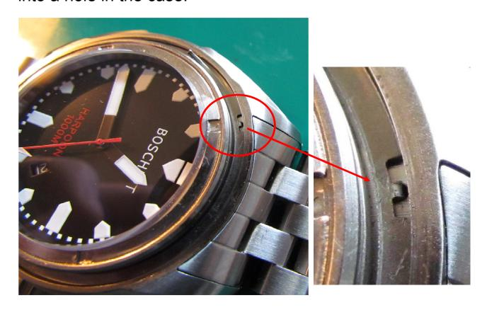
Place the ceramic bezel on the case and push down. You will hear it "snap" on. Check to make sure it properly rotates.
