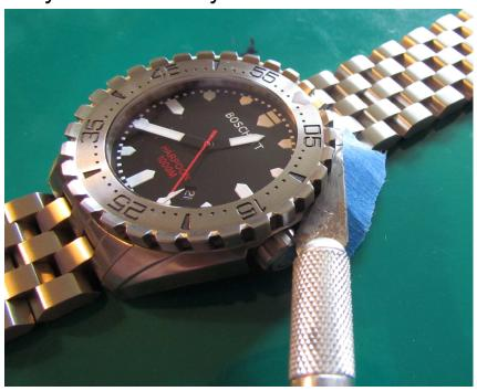
Note the position of the stainless steel octagonal spring and the white retension gasket on the underside of the bezel. They should be installed in the same manner on the ceramic bezel. The white gasket should be installed first, then the SS spring on top.
